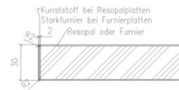
**Plate D:** 30 mm thick, 28 mm thick high-quality multi-layer plywood plate E1, top surface optionally covered with HPL plastic or wood veneer according to the BRUNE® collection. Lower surface white HPL or beech veneer. Edge with solid beechwood edge band, smooth finish, 9 mm thick.
